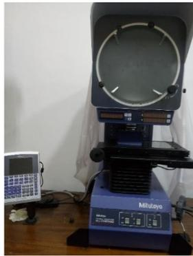
Gambar 1.1 Alat ukur profile projector
